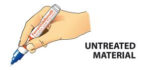
If the liquid splits into droplets in less than 2 seconds, the sample **has not undergone corona treatment**. Its wettability is less than **38 dyne/cm**.
